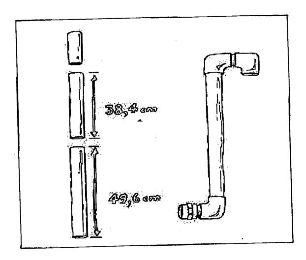
5. With another 5 cm section from the leftover pipe glue the female connector (adaptor) to the lower end of the outlet pipe (the end with just one elbow joint).
